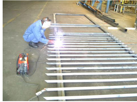
Fabrication of steel gates for Rand Water.
